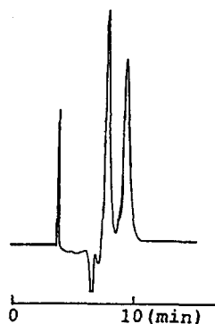
Fig. 5. Enantiomeric separation of racemic norphenylephrine on phase I. Chromatographic conditions as in Table III.
